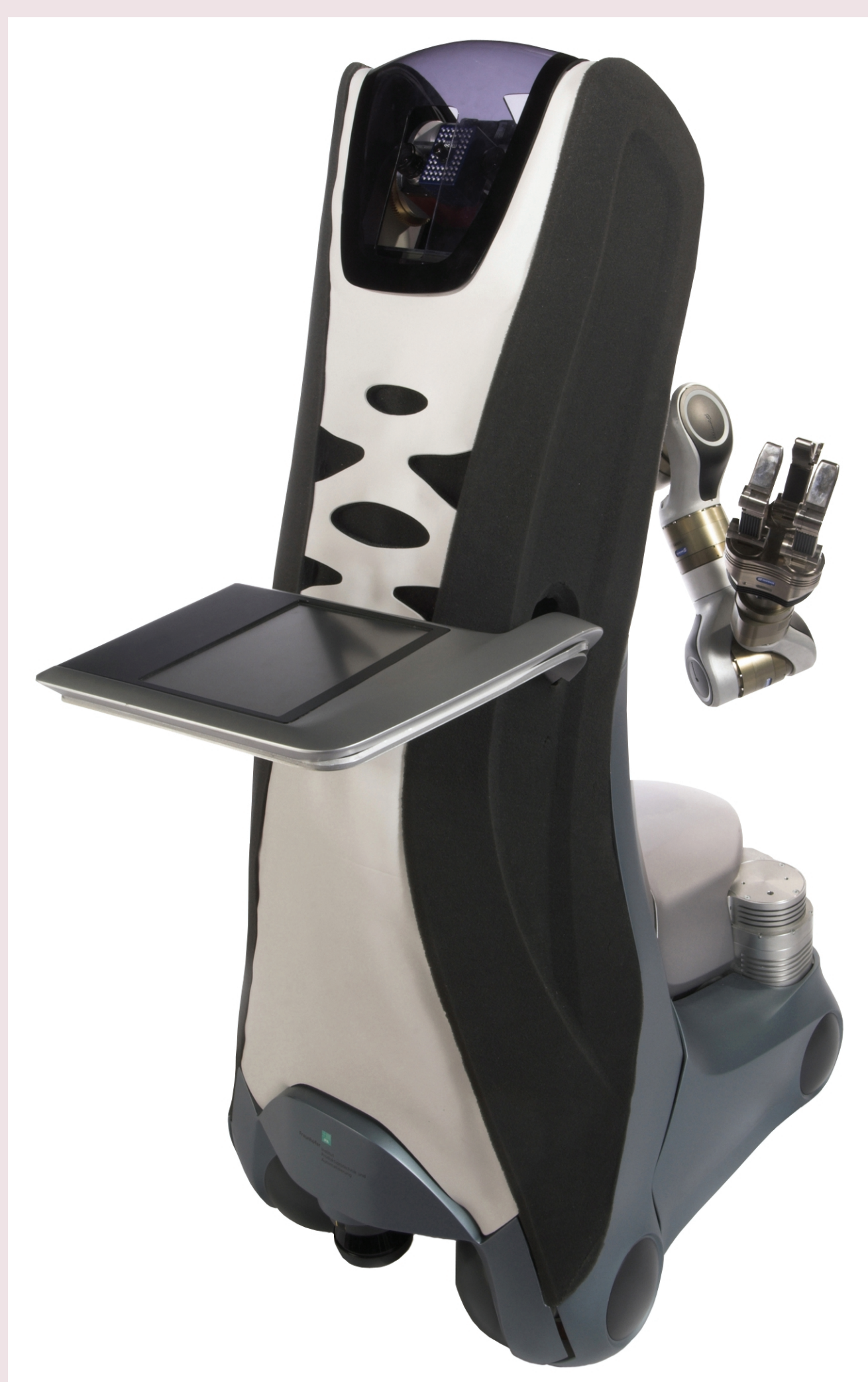
Figure 1: Care-O-bot® 3 – Mobile Robot Assistant, Fraunhofer IPA, Stuttgart
