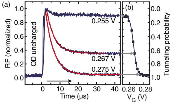
FIG. 2. (a) Measured time-resolved RF signal of the exciton transition (trion out of resonance) for three different charging voltages  $V_2$  (red lines are exponential fits, used to obtain relaxation rates). (b) Normalized RF signal at  $t = 40 \mu\text{s}$  as a function of gate voltage.
