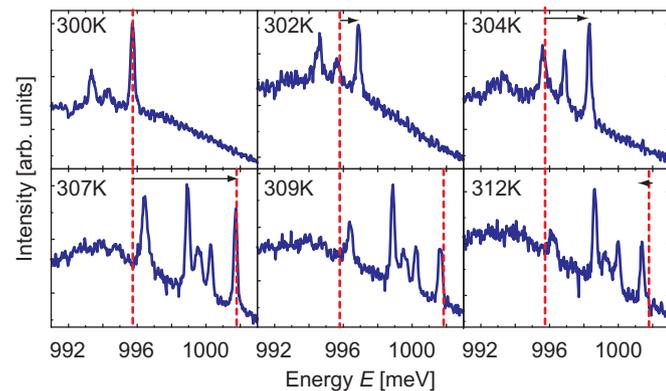
Fig. 4. Temperature dependent mode shift induced by reorientation of the liquid crystal.
