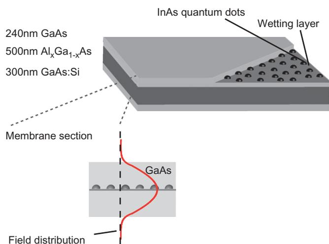
Fig. 1. Sample material for microdisk fabrication.
