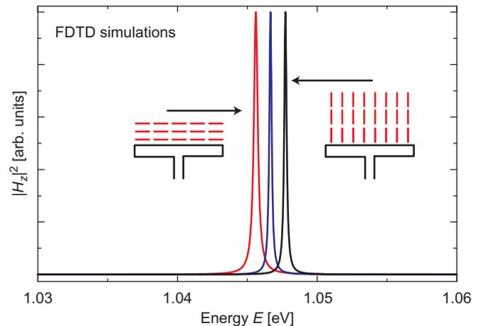
Fig. 6. Finite differences time-domain simulations of the microdisk devices embedded in an anisotropic dielectric material showing a mode shift induced by the orientation of the liquid crystal.
