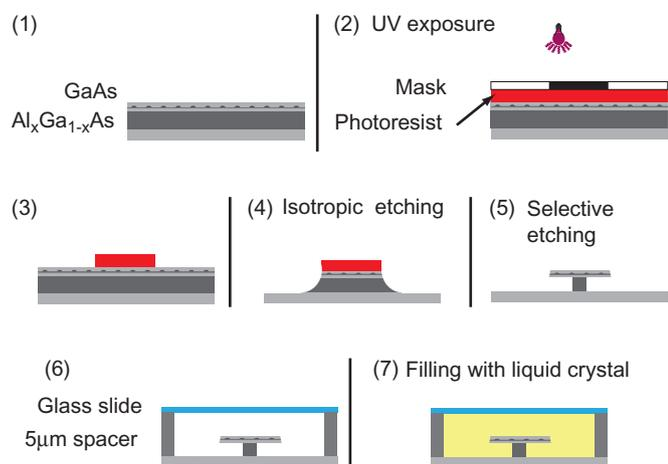
Fig. 2. Processing sequence for the formation of LC-filled microdisks.
