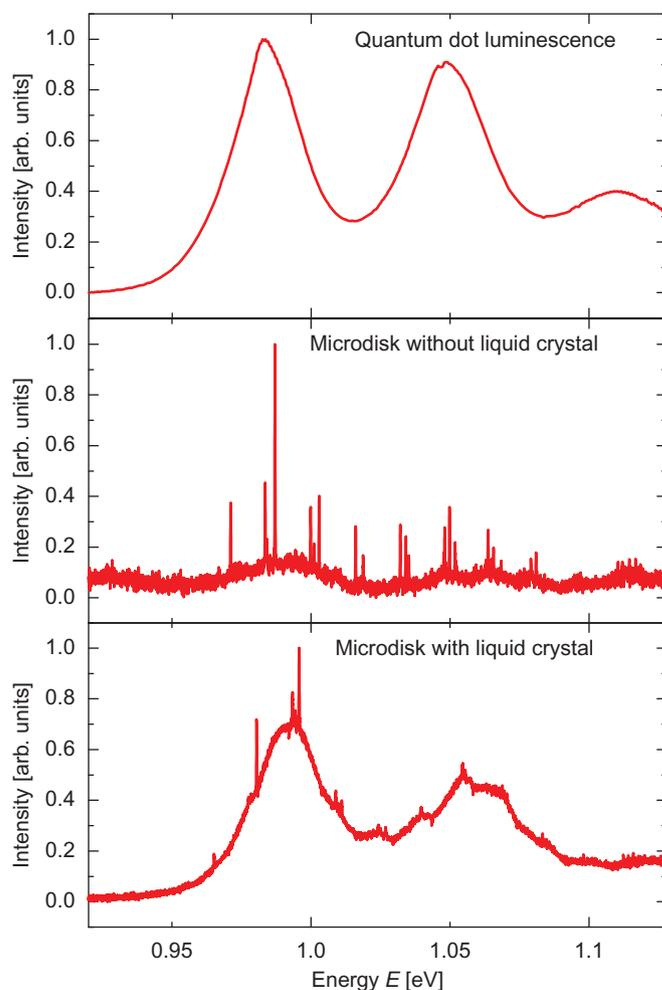
Fig. 3. PL spectra of (top) quantum dots at 300K before sample fabrication, (middle) microdisk (with QDs) at 300K and (bottom) microdisk immersed in liquid crystal.
