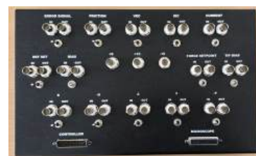
Figure 7.1: Photograph of the auxiliary data acquisition unit used to access internal signals of the SPM 5500. Via BNC connectors, the microscope can be directly connected to a digital storage oscilloscope (e.g., MephistoScope) for external signal readout.
