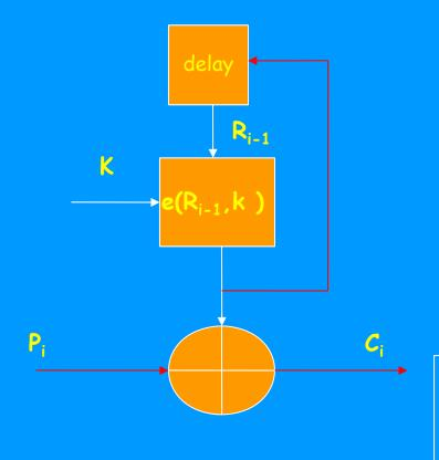
$C_i = P_i \oplus e(R_{i-1}, k)$  $P_i = C_i \oplus e(R_{i-1}, k)$  R<sub>0</sub> given
