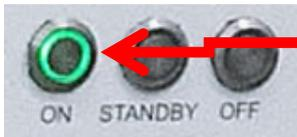
2. Check if the SEM is switched on. The green „On“ light must be on – if not switch it on by pressing the knob.
