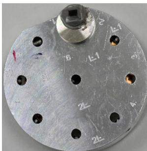
The stubs are mounted here by turning the screws on the side of the dish (If the holder cannot be found it most probably still is in the SEM and has to be retracted from there – the necessary procedure for doing this is explained later on page 5)
