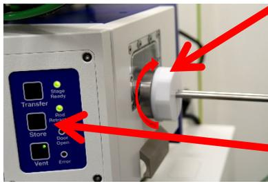
Then turn the white ring clockwise in a way that the docking position is reached. The image shows the situation with the holder in correct docking position.
