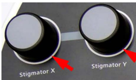
The better the accuracy of wobbling the better the image quality. After finishing the wobbling it is necessary to readjust the focus (potentiometer 11). Next is the correction of the stigmatism with help of the two Stigmator potentiometers shown on the left (2 & 3) which are turned while regarding the live image. The
