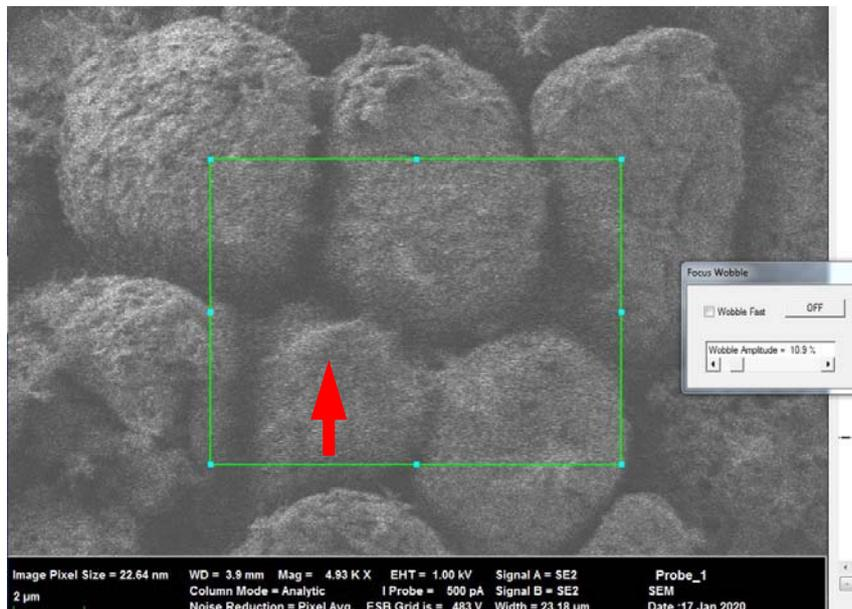
in which the wobbling is active. You can adapt the size of the borders when touching them with the mouse while clicking. The small popping up Focus wobble window allows you to manipulate the frequency and amplitude of the wobbler (best is to try with low values). The aim is to completely reduce the movement to
