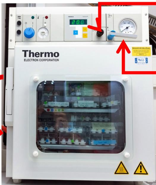
After this perform the reversed procedure to restart the vacuum in the storage: close the inner glass door, put the on the left of the door in upright position while pressing the door tightly.
