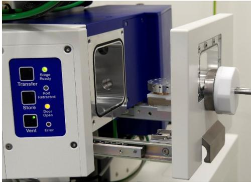
The handle of the door now unlocks and you can open the door now WITH GLOVES. Hold the sample plate while turning the holder counter clockwise und detach it.
