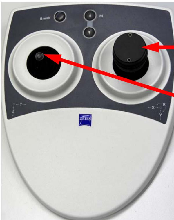
You can move the sample plate with help of the joystick navigation which influences the position of the sample:
