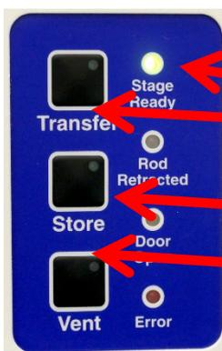
Now look in the camera window of the software and drive the stage to the exchange position. After this you see a flashing of the „Stage Ready“ diode on the lock of the SEM.
