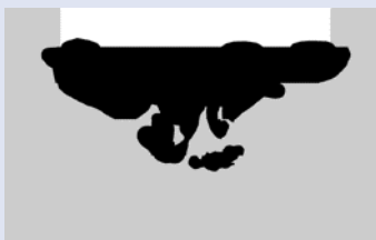
Simulated cavitation bubble field under a sonotrode
