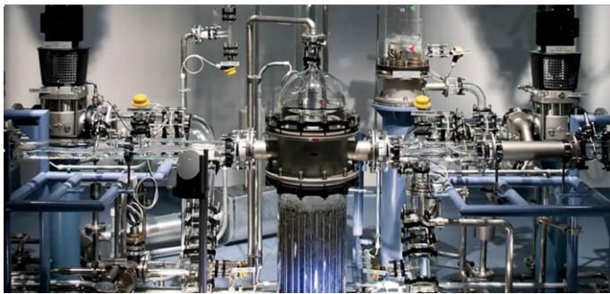
Glass model of a pressurized water reactor (PWR) ©Gesellschaft für Simulatorschulung mbH
