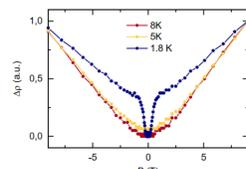
Comparison of relative resistivity-change versus magnetic field at three different temperatures (taken from [1])
