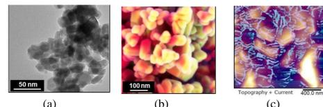
(a) Transmission Electron Microscopy (TEM) (b) Scanning Electron Microscopy (SEM) and (c) Atomic Force Microscopy (AFM) images of Bi<sub>2</sub>Te<sub>3</sub> nanoparticles (taken from [1])
