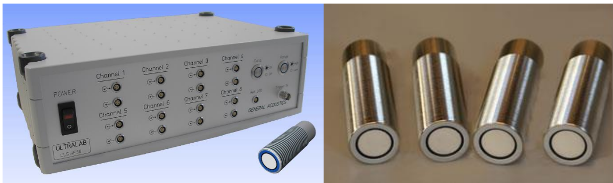
Abbildung 3 UltraLab Controller (links), UltraLab Sensoren (rechts) (Homepage General Acoustics)
