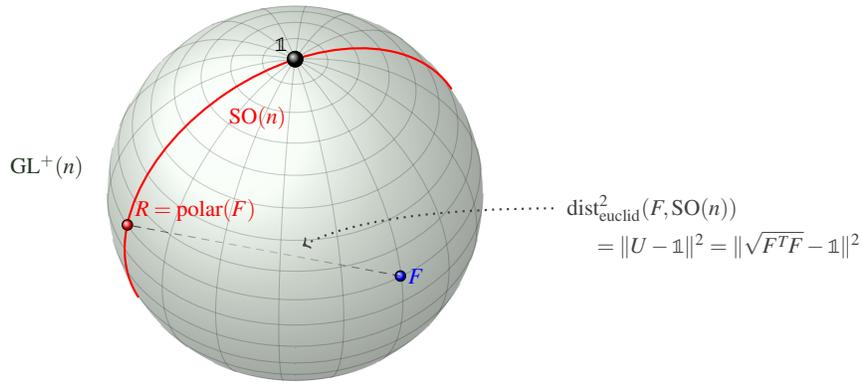
Fig. 1: The Euclidean distance as an extrinsic measure on  $\text{GL}^+(n)$ ; note that the representation of the manifold  $\text{GL}^+(n)$  as a sphere only serves to demonstrate the necessity of an intrinsic distance measure and does not reflect the actual topological properties of  $\text{GL}^+(n)$ .
