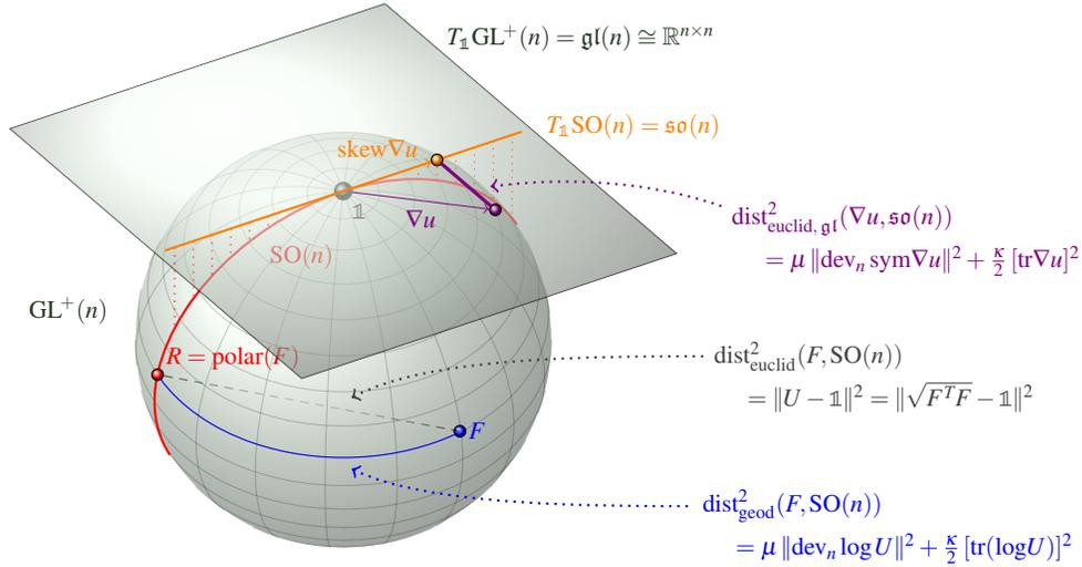
Fig. 4: The isotropic Hencky energy of  $F$  measures the geodesic distance between  $F$  and  $SO(n)$ . The linear Euclidean strain measure is obtained via linearization of the tangent space  $\mathfrak{gl}(n)$  at  $\mathbb{1}$ .
